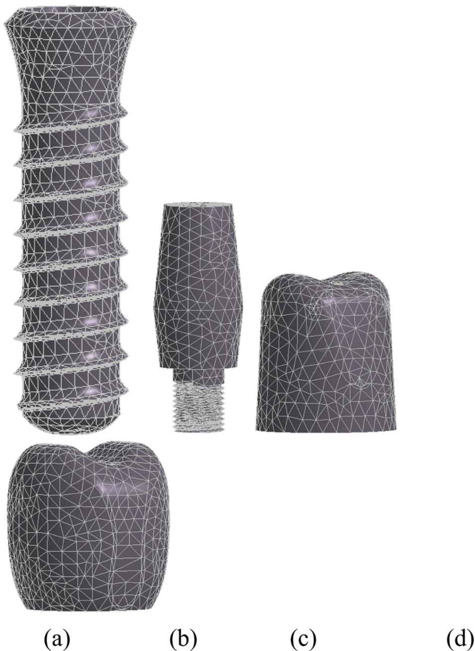
Fig. 3. FEM models of implant (a), abutment (b), metal framework (c) and occlusal material (d).
