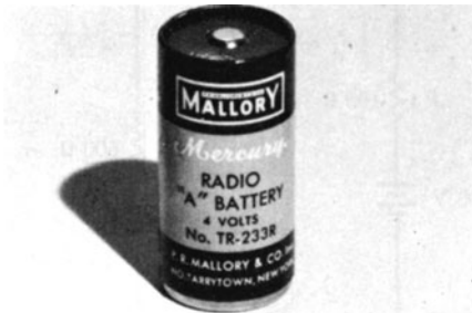
Fig. 6-10 A typical mercury battery. (Courtesy NRI Schools.)
