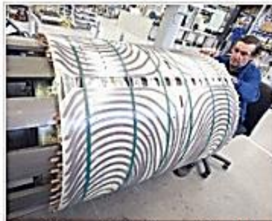
Gradient coil with thin metallic strips being applied in a fingerprint pattern to a former (courtesy Siemens)
